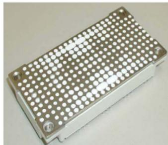
Fig. 6: Print image after blade squeezing
