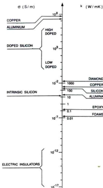
Figure 1: Comparison between electrical and thermal conductivities
