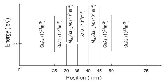
Fig. 1. The double barrier resonant tunneling structure.
