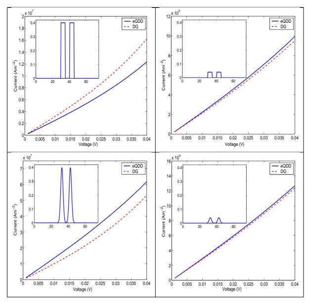
Fig. 12. Influence of the shape and the height of the double barrier on the Current-Voltage characteristics for the eQDD and DG models.
