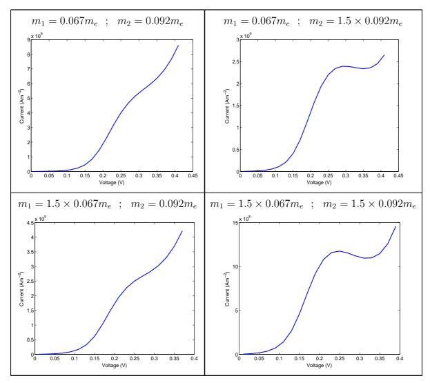
Fig. 6. Influence of the effective mass on the IV curve,  $m_1$  being the mass outside the barriers, and  $m_2$  being the mass inside.
