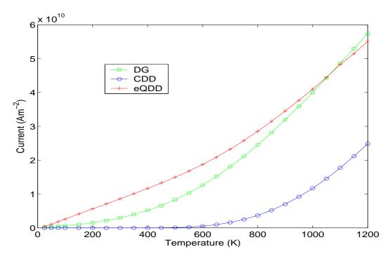
Fig. 13. Current-Temperature curve (applied bias: 0.2V).
