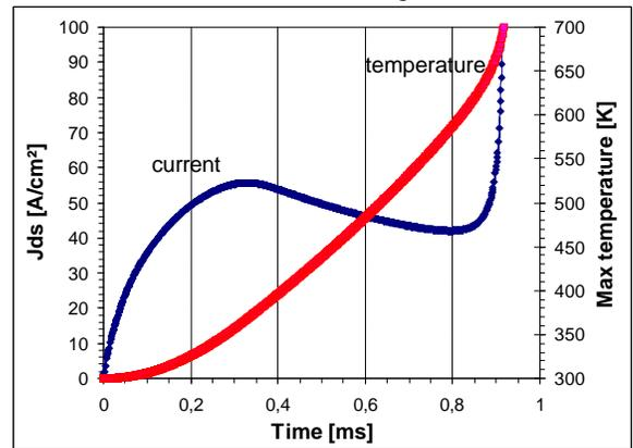
**Figure IV-3: Thermal run-away of a silicon current limiting device (same  $V_{DS}$ -ramp condition and thermal boundary conditions as for the SiC device figure IV-1).**
