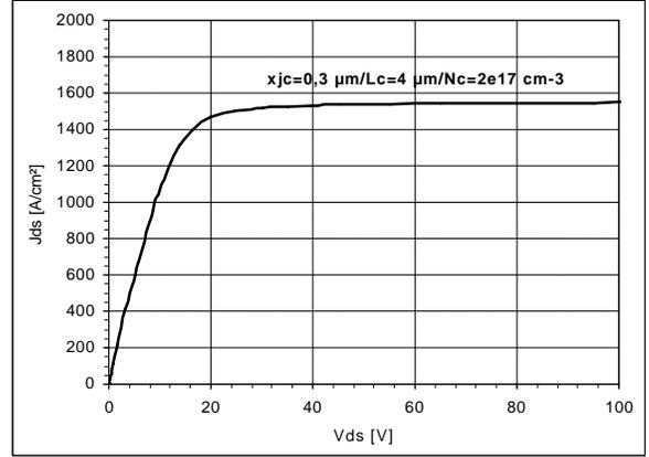
Figure III-2: I-V curve at  $T=300\text{K}$  (channel depth= $0,3 \mu\text{m}$ ; channel length= $4 \mu\text{m}$ ; channel doping level= $2 \cdot 10^{17} \text{cm}^{-3}$ ,  $L_{intercell}=10 \mu\text{m}$ )
