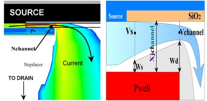
Figure III-3: Left picture: 2D mapping of the current inside the device near the channel region. Right picture: simplified current path in the channel.
