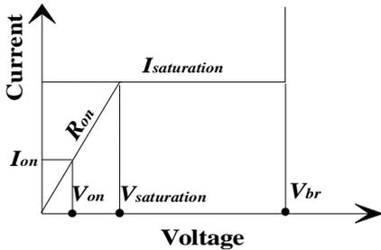
Figure III-1: typical I-V characteristic of a current limiting device.
