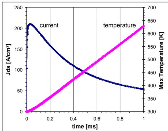
**Figure IV-1: Current density and the maximum temperature inside the device versus time during a 500V/1ms  $V_{DS}$ -ramp. (channel depth=0,2  $\mu\text{m}$ ; channel length=4  $\mu\text{m}$ ; doping level= $2 \cdot 10^{17} \text{ cm}^{-3}$ ,  $T_A=300\text{K}$ ,  $R_{TH}=0.5 \text{ K.cm}^2/\text{W}$  at the backside,  $R_{TH}=\infty$  at the topside).**
