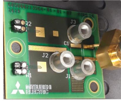
Fig. 8: Close-up on the PCB under test (Dimensions: 35mm\*45mm) and the tip of the Keysight 42941A probe placed across the decoupling capacitor footprint to measure the power loop impedance (decoupling capacitors not mounted).
