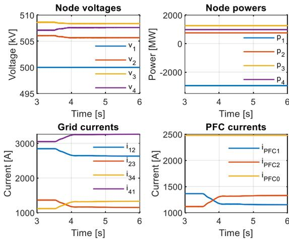
Fig. 21 Bypass sequence simulation results.
