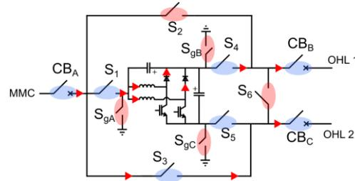
Fig. 8. Insertion sequence: step 4.  $S_2$  open.
