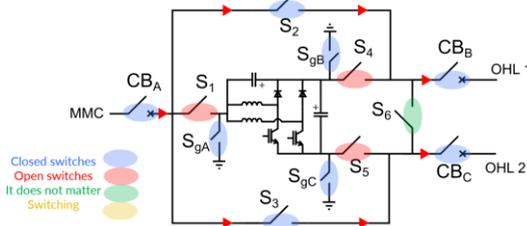
Fig. 5. Insertion sequence: step 1. PFC bypassed and grounded.
