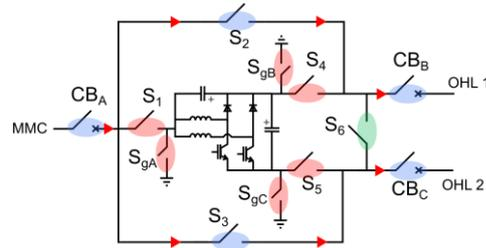
Fig. 6. Insertion sequence: step 2. PFC ungrounded.
