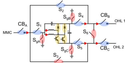
Fig. 12. Bypass sequence: step 2.  $S_2$  closed.
