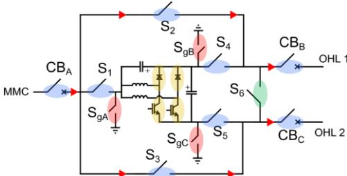
Fig. 13. Bypass sequence: step 3.  $S_3$  close, PFC bypassed
