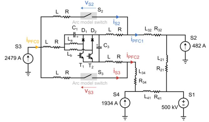
Fig. 18. Model of the PFC and HVDC during the insertion sequence in EMT.
