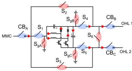
Fig. 9. Insertion sequence: step 5.  $S_3$  open.
