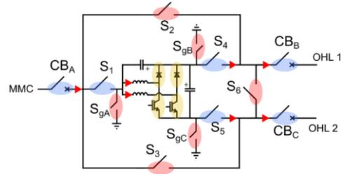
Fig. 10. Insertion sequence: step 6. PFC in operation.
