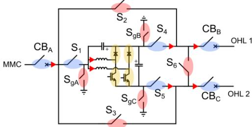
Fig. 11. Insertion sequence: step 1. PFC in operation.
