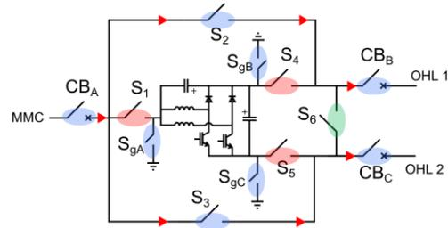
Fig. 16. Bypass sequence: step 6. PFC grounded.
