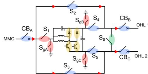
Fig. 14. Bypass sequence: step 4.  $S_1$  open
