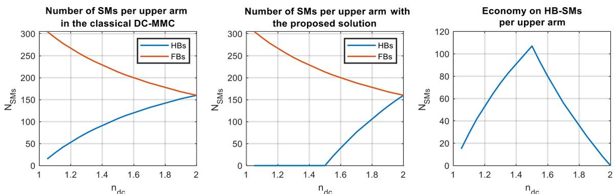
Fig. 4: Number of SMs per upper arm on the classical DC-MMC, in the proposed solution and the economy of HB-SMs for the proposed solution. A DC system voltage of  $V_H = 640 \text{ kV}$  and SM voltage of  $V_{SM} = 2 \text{ kV}$  were assumed as an example.
