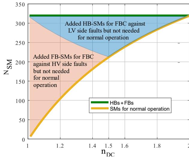
Fig. 2: Number of SMs required on each upper arm for normal operation and to provide FBC. A DC system voltage of  $V_H = 640 \text{ kV}$  and SM voltage of  $V_{SM} = 2 \text{ kV}$  were assumed as an example.
