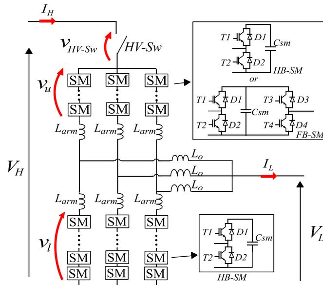
Fig. 3: DC-MMC with external HV-Sw to provide FBC against LV faults.
