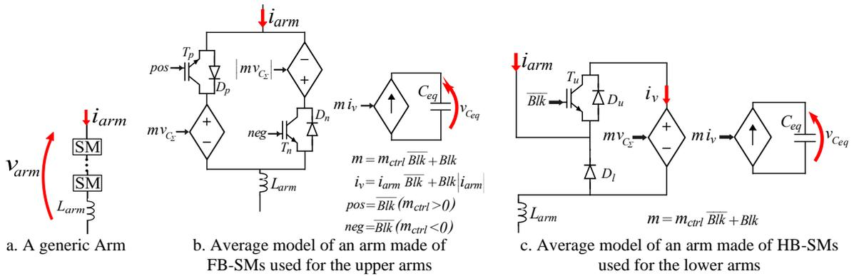
Fig. 5: Simulation models of an arm used to model the DC-MMC.
